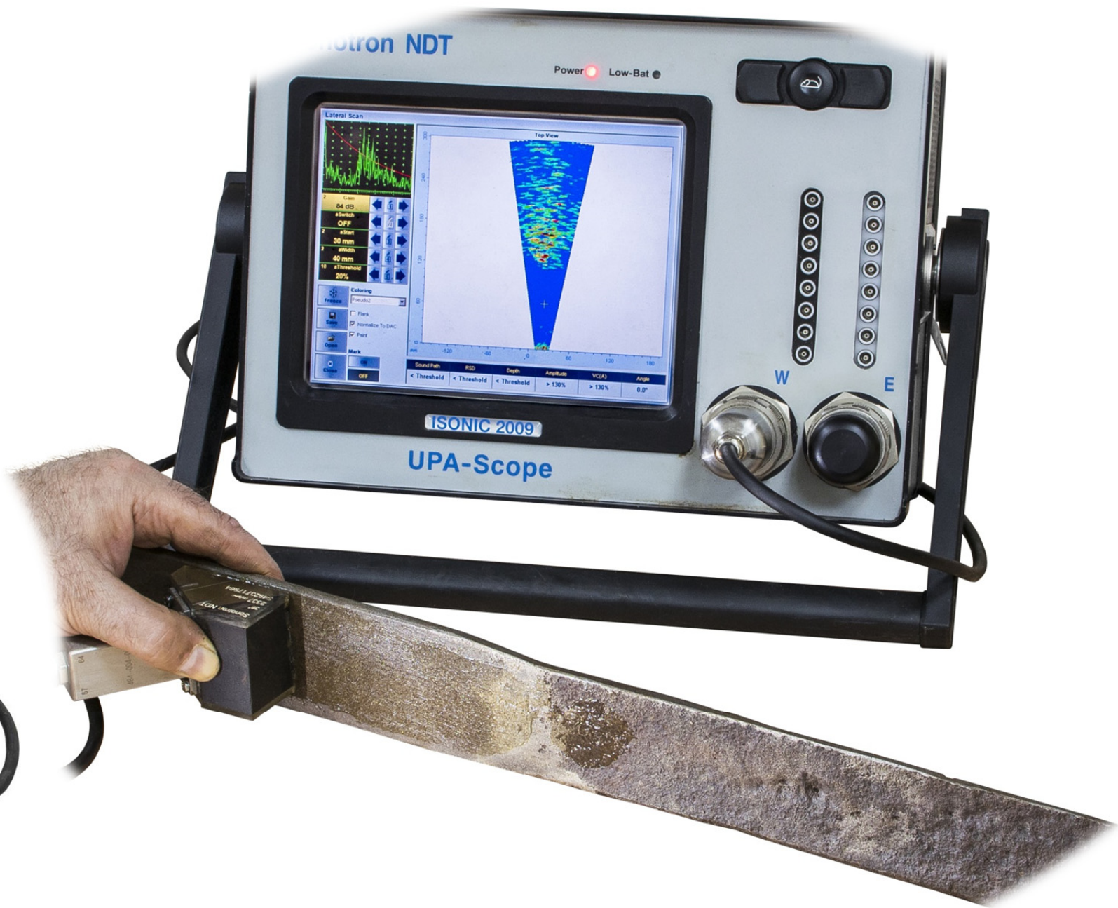
Detection of the corrosion in the area of air to soil interface
