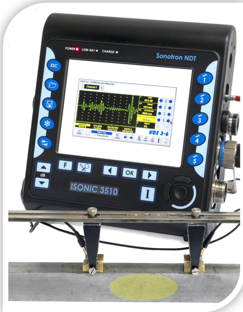
TOFD A-Scan for the vertical planar defect obtained with the use of a pair of regular probes connected to the conventional channel of ISONIC 3510 instrument (UDS 3-6 Pulser Receiver)
