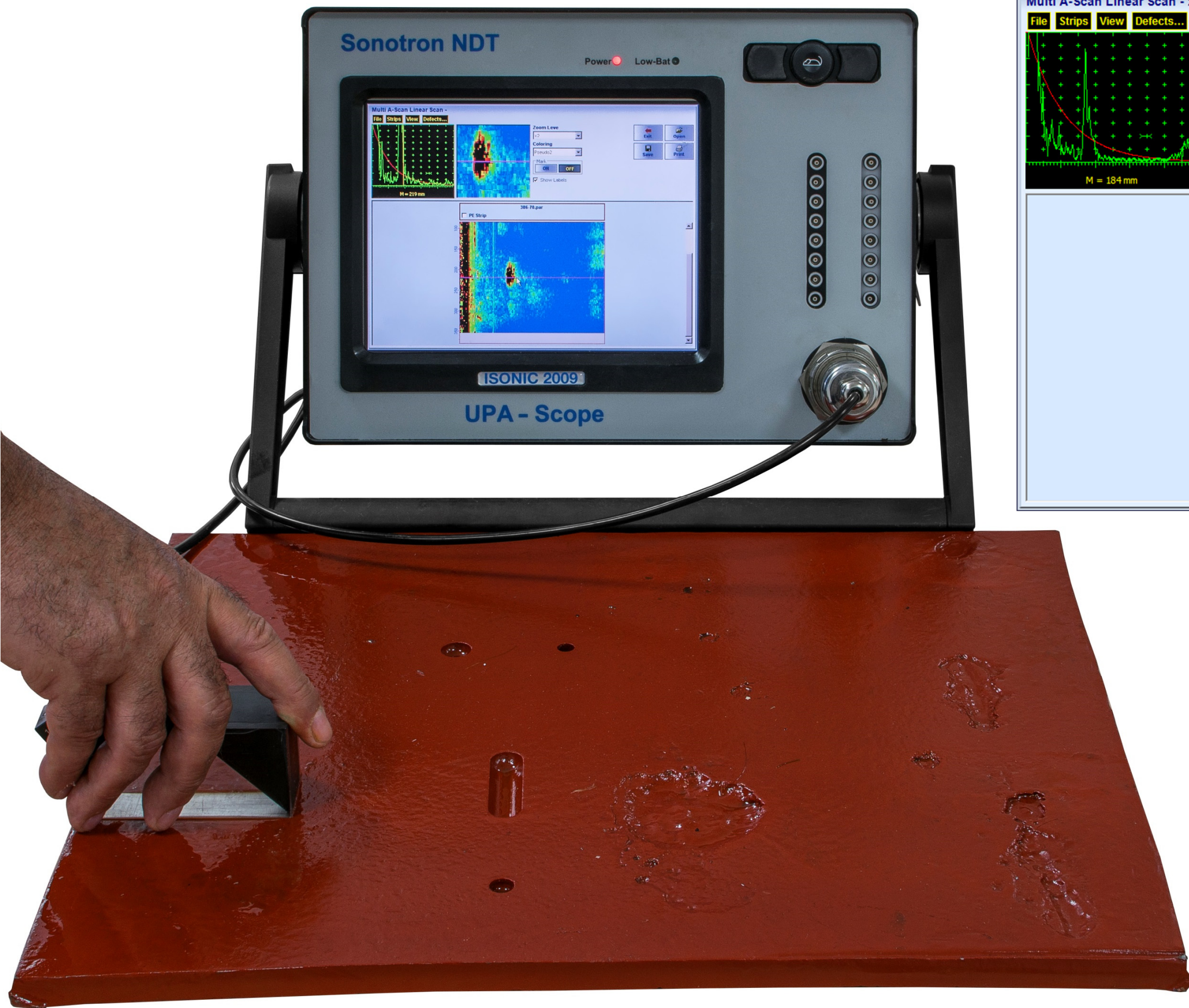
SRUT Guided Wave Inspection with use of PA probe and Recording a single MAP STRIP
