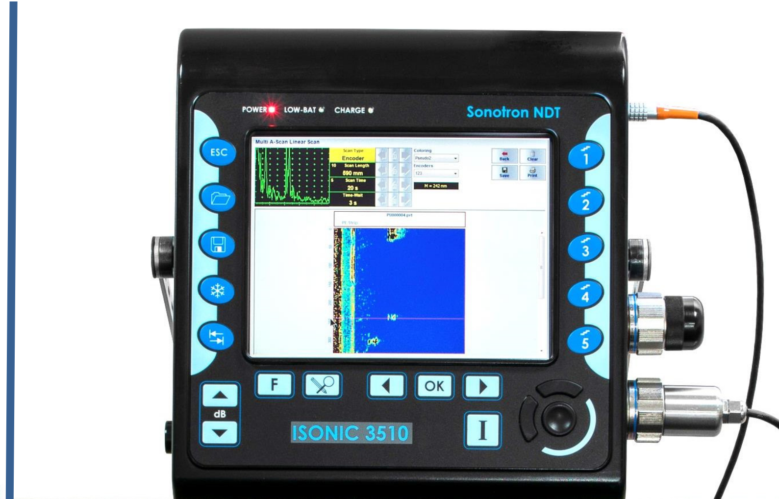
Pipe wall map obtained through the scanning
