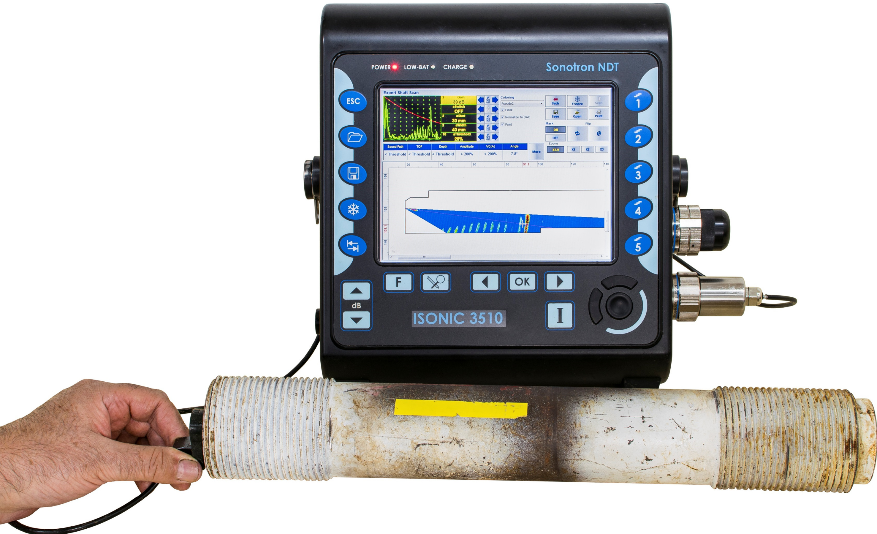
Inspection of Hollow Stud Bolts
