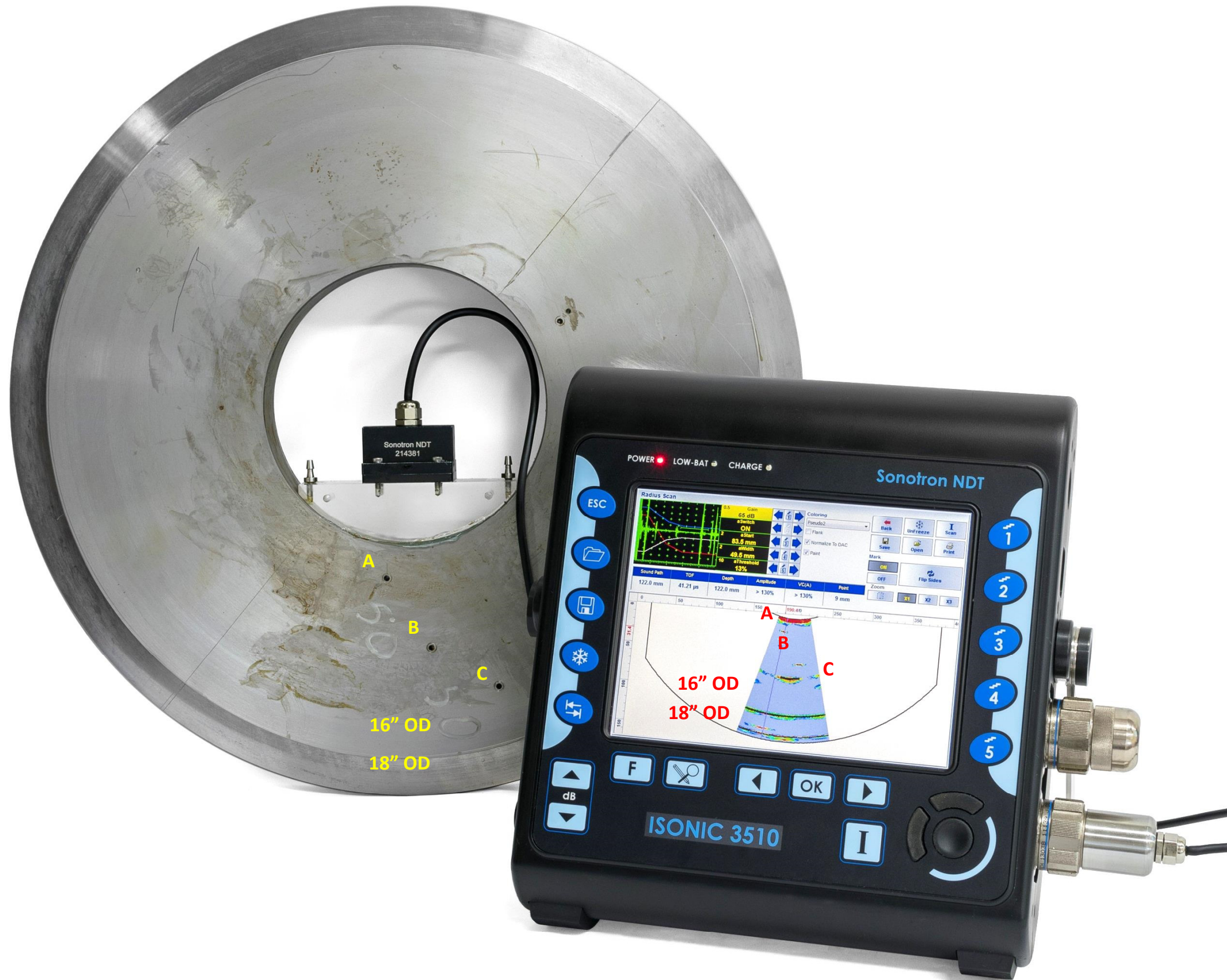
Calibration Block / PDB for the shaft inspection
