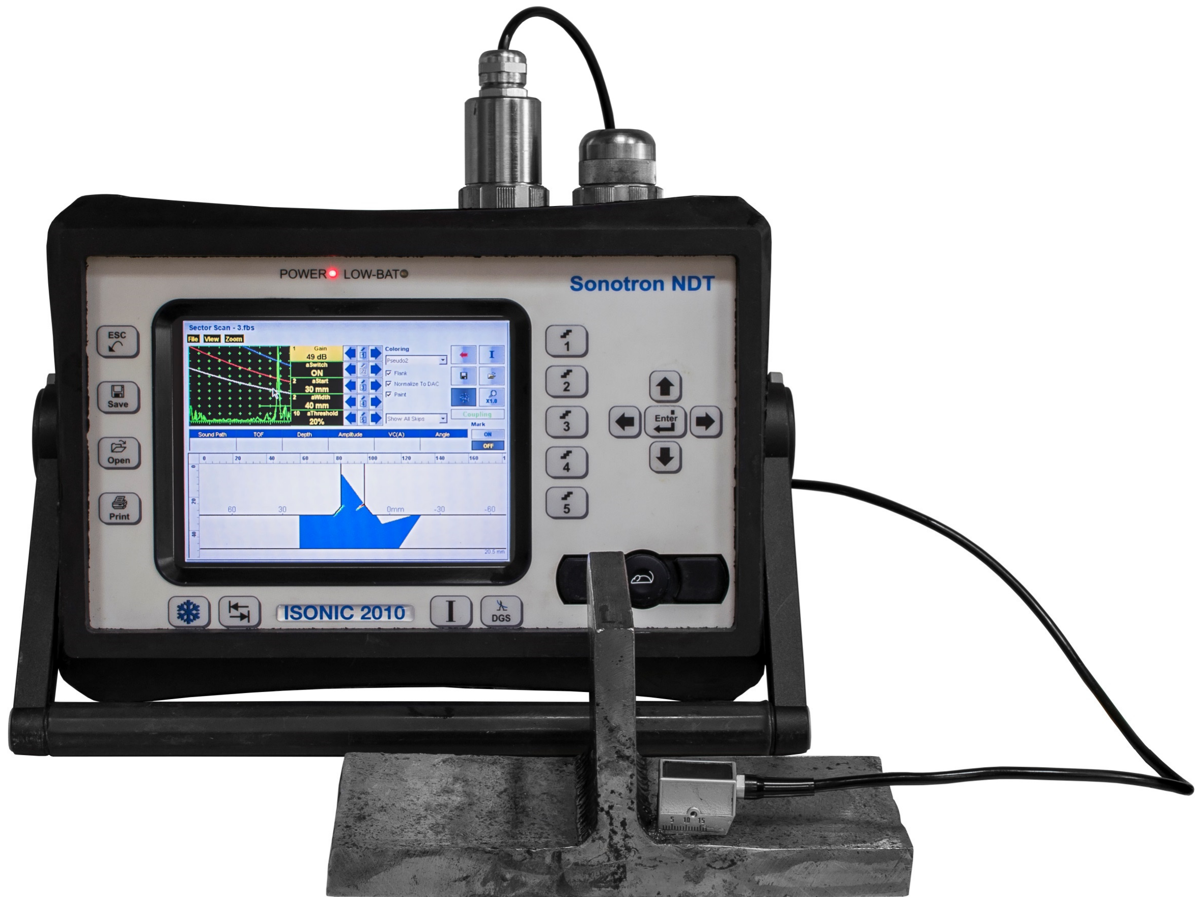
Shear wave inspection of the fillet weld – probe placement on the inner side of the flange
