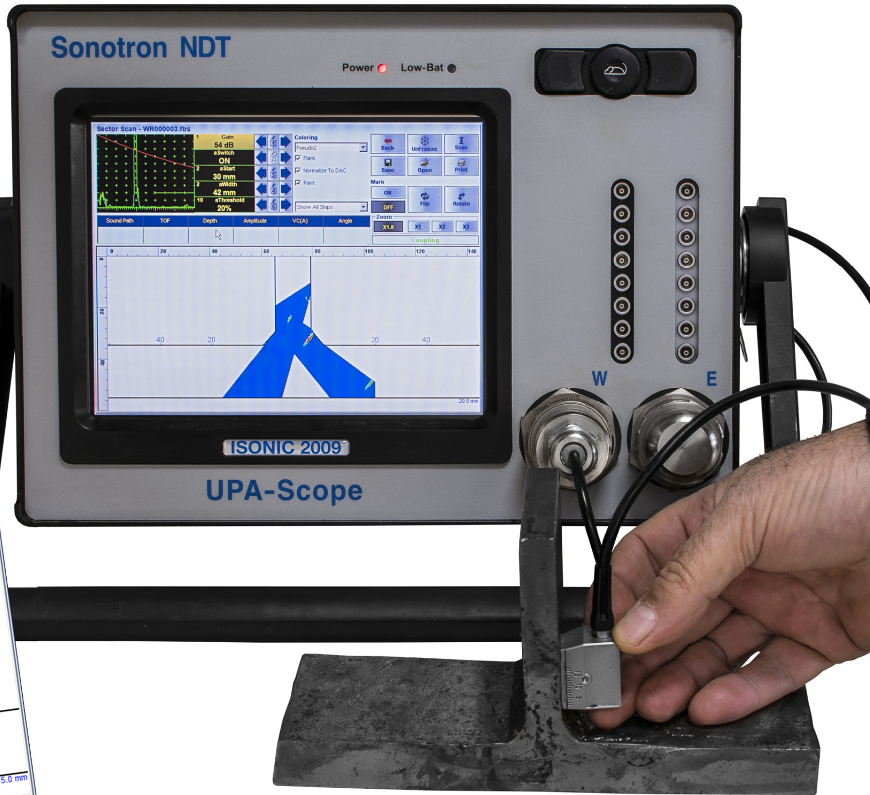
Shear wave inspection of the fillet weld – probe placement on the web
