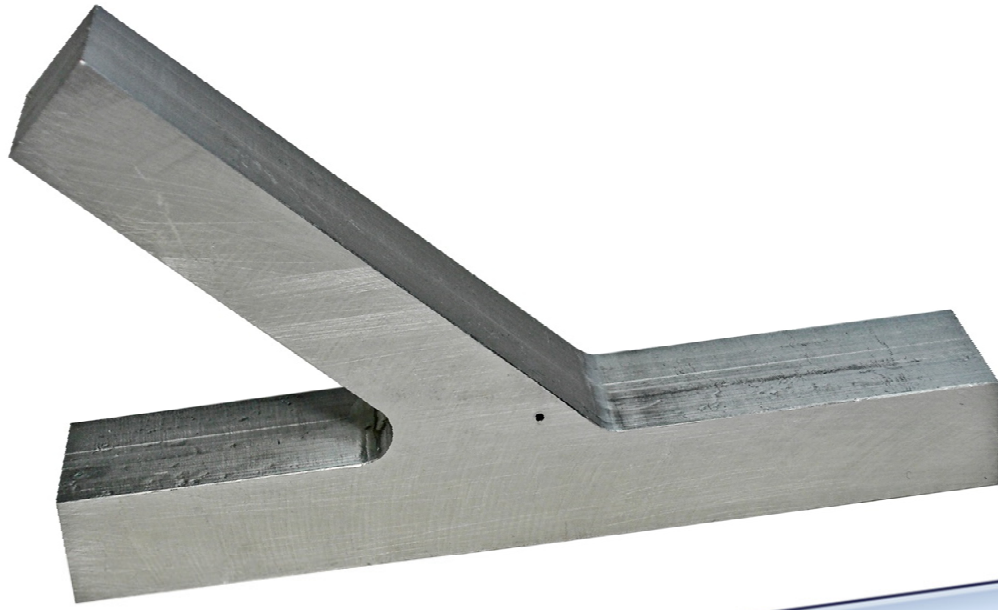
Shear wave inspection of the skewed fillet weld (performance demonstration block) – probe placement on the inner side of the flange
