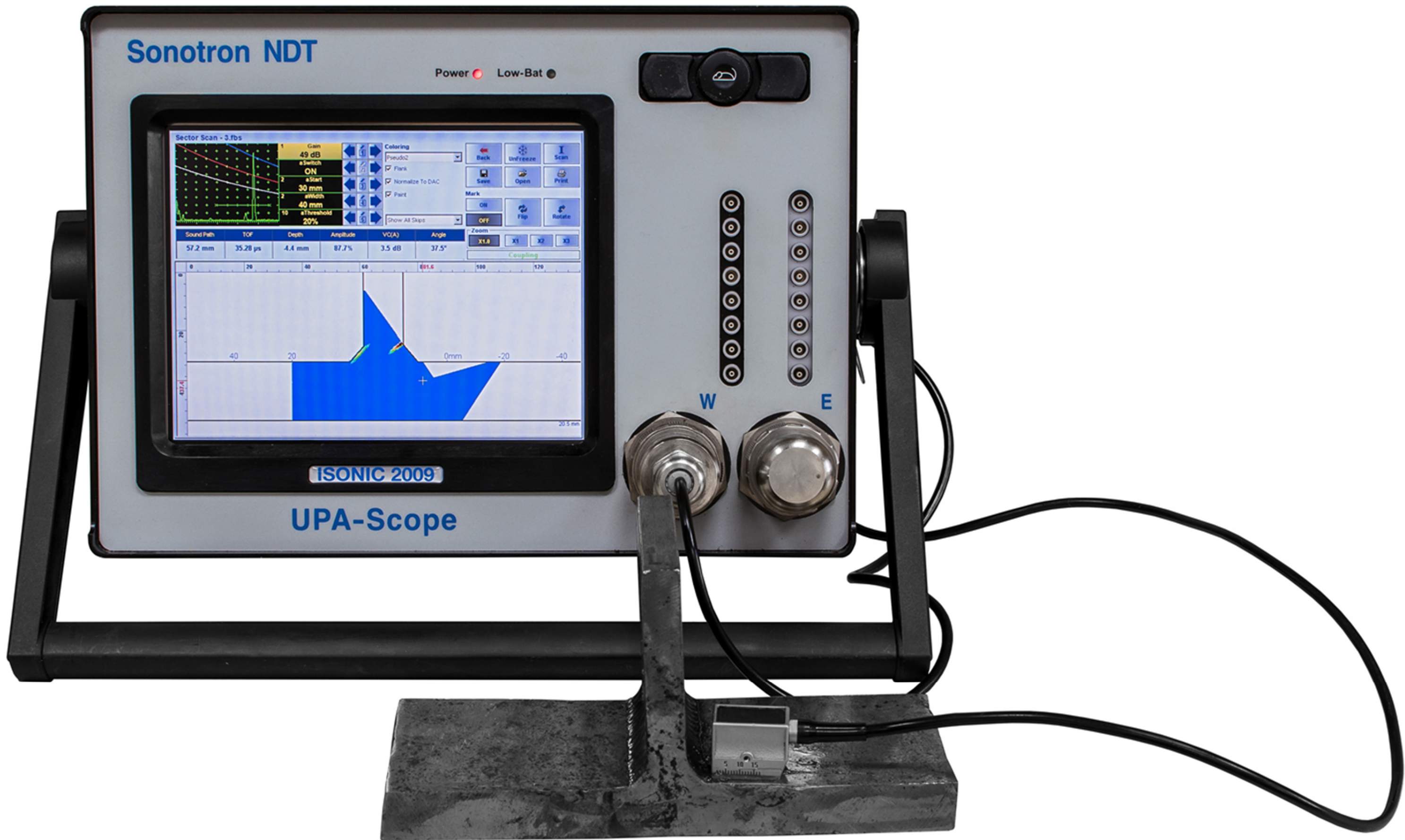
Shear wave inspection of the fillet weld – probe placement on the inner side of the flange
