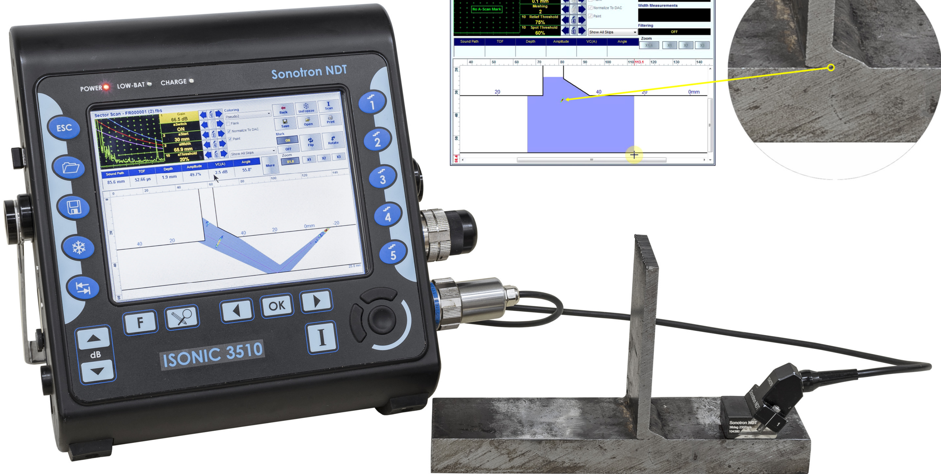
Determining the partial penetration of the one side welded fillet
