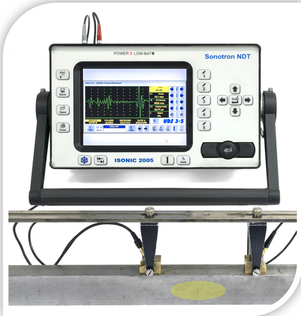
TOFD A-Scan for the vertical planar defect obtained with the use of a pair of regular probes connected to ISONIC 2005 instrument (UDS 3-5 Pulser Receiver)
