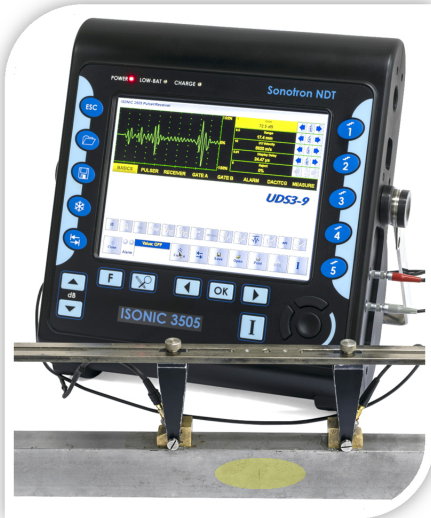
TOFD A-Scan for the vertical planar defect obtained with the use of a pair of regular probes connected to ISONIC 3505 instrument (UDS 3-9 Pulser Receiver)
