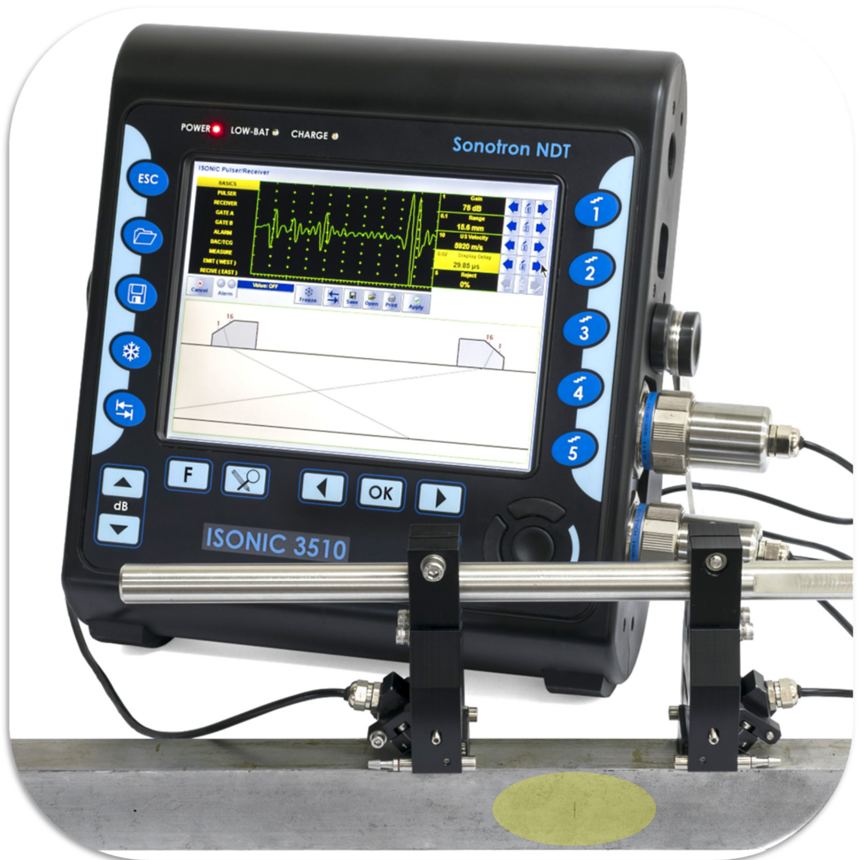
TOFD A-Scan obtained on the vertical planar defect with use of a pair of PA probes of the same frequency as regular TOFD probes
