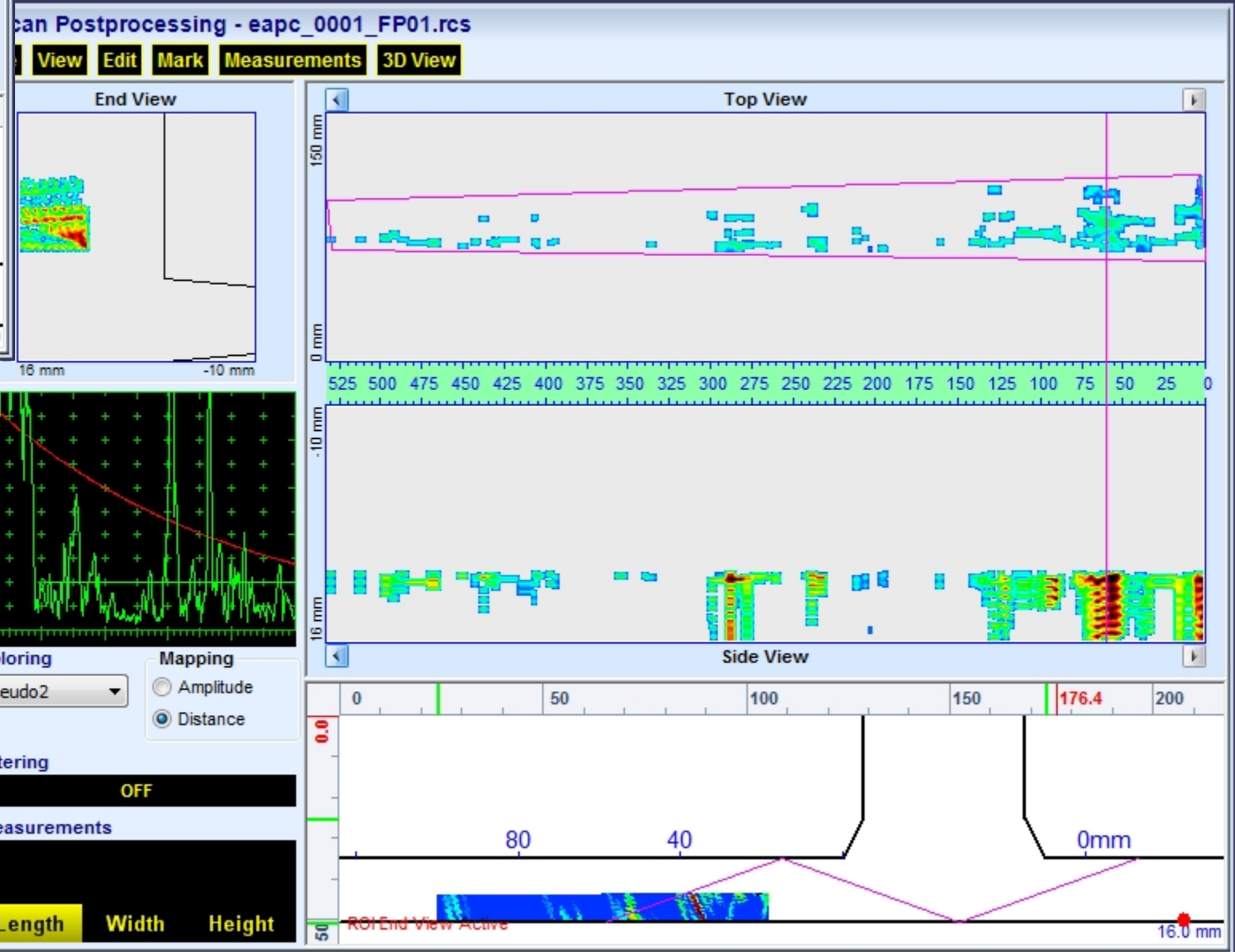
C-Scan (Top View), Side View, End View Data for the scattered corrosion inside the tank at the soil side
