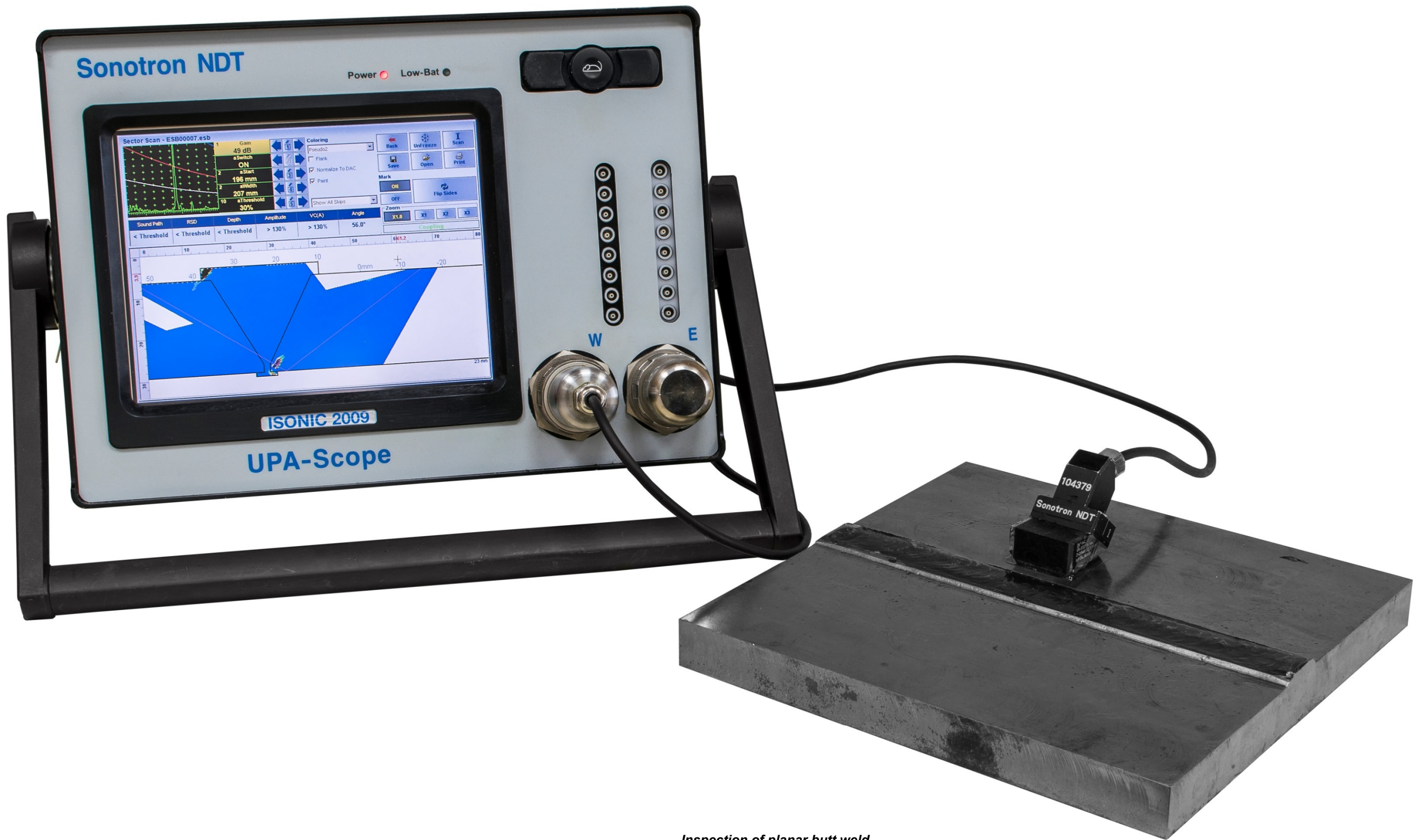
Inspection of planar butt weld
