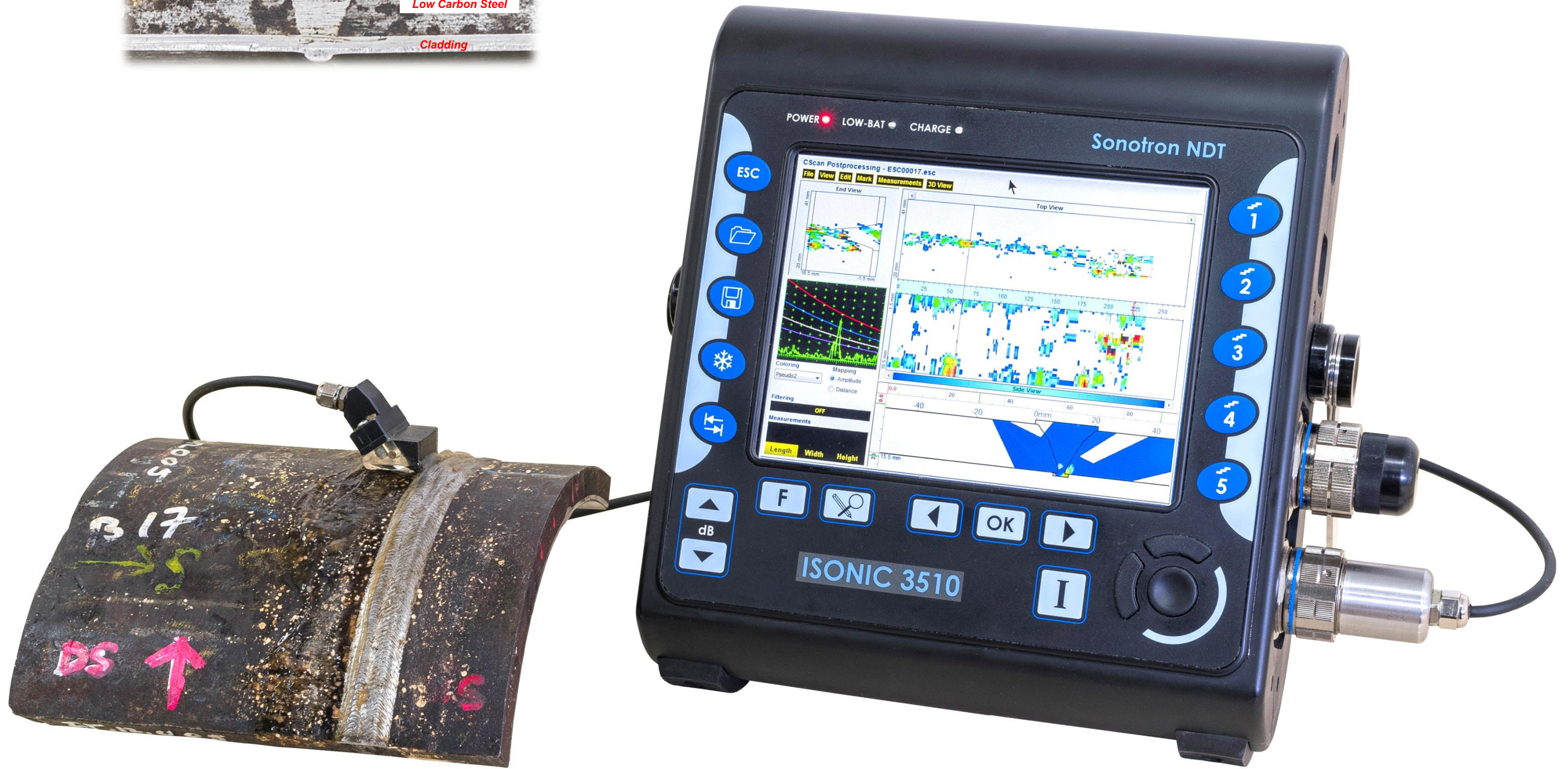
Inspection of stainless steel circumferential butt weld between cladded pipes – shear waves out of small aperture 2 MHz probe
