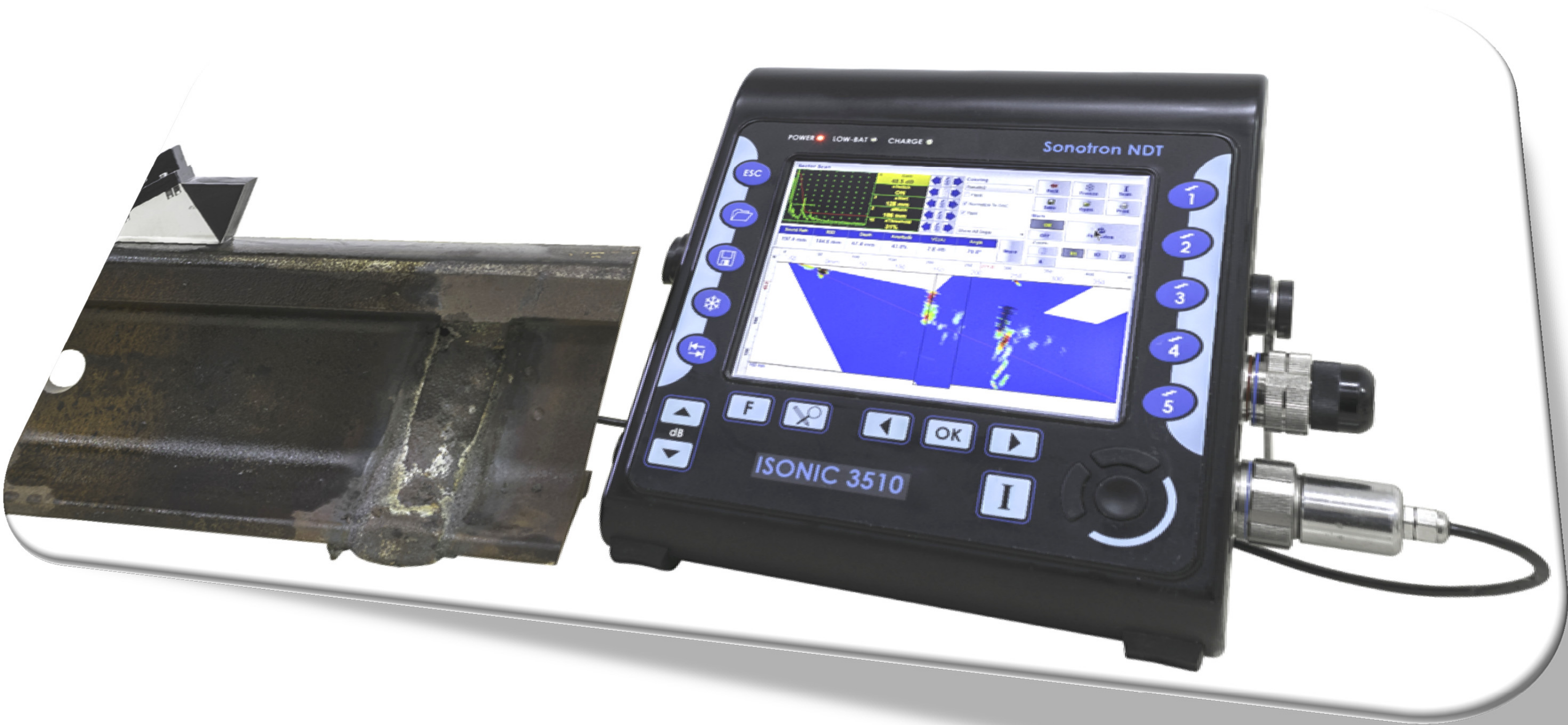
Inspection of the rail thermite welds
