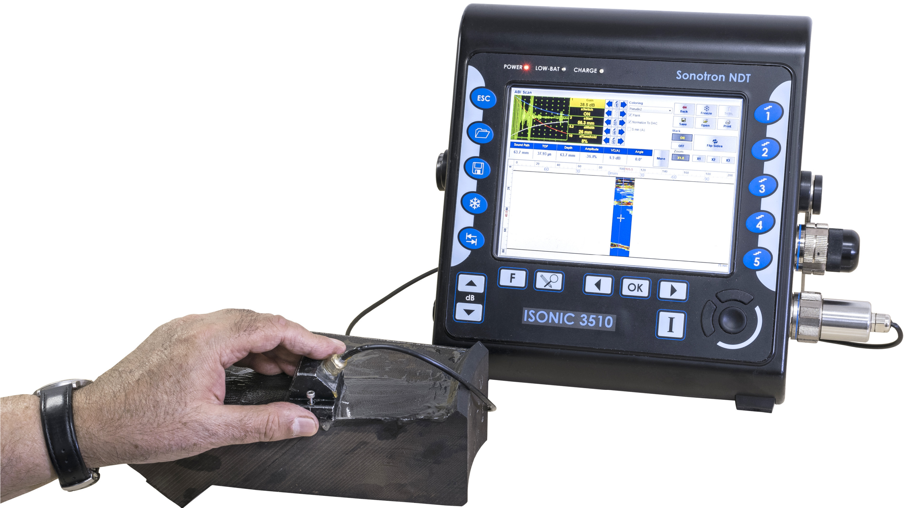
Inspection of heavy thickness CFRP part Compression wave B-Scan coverage
