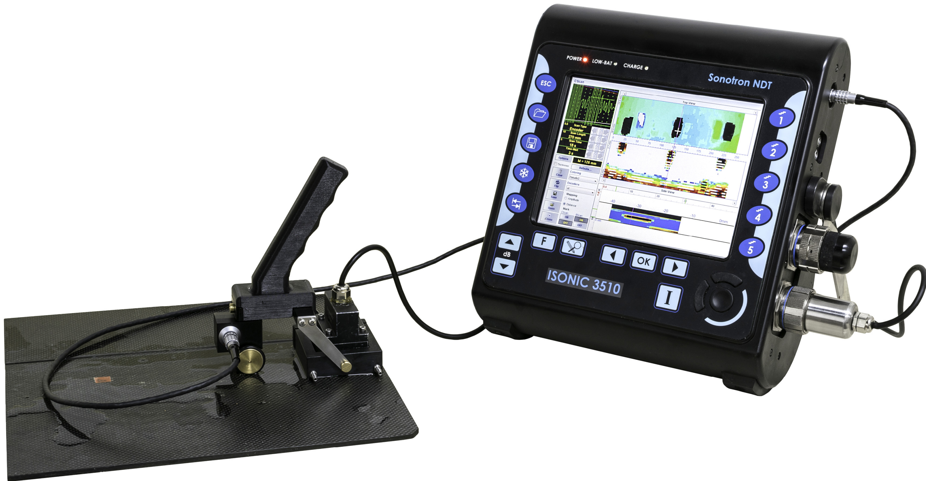
Inspection of CFRP plate Compression wave B-Scan coverage with C-Scan imaging and recording
