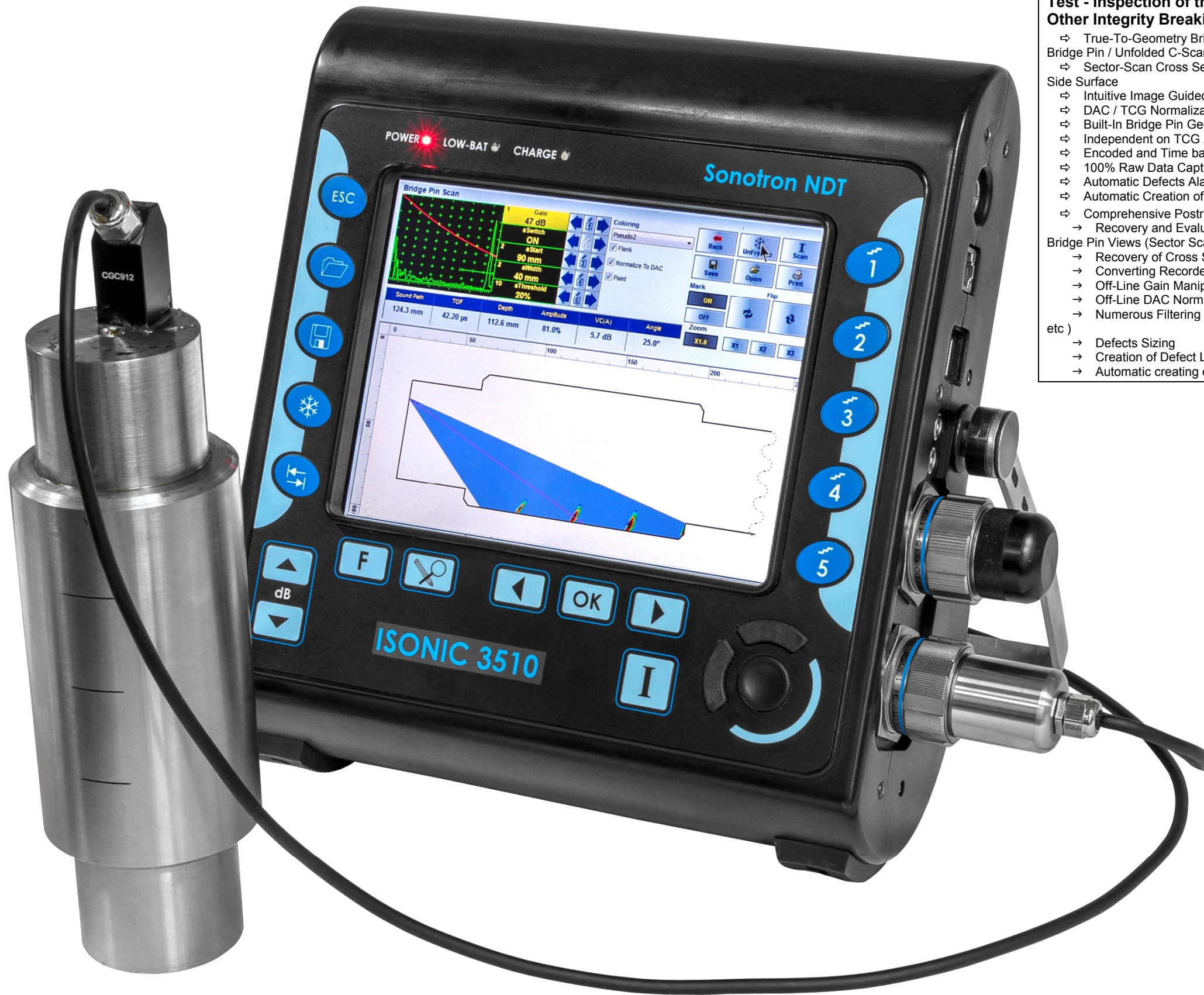
Inspection of the bridge hanger pins – calibration / performance demonstration block
