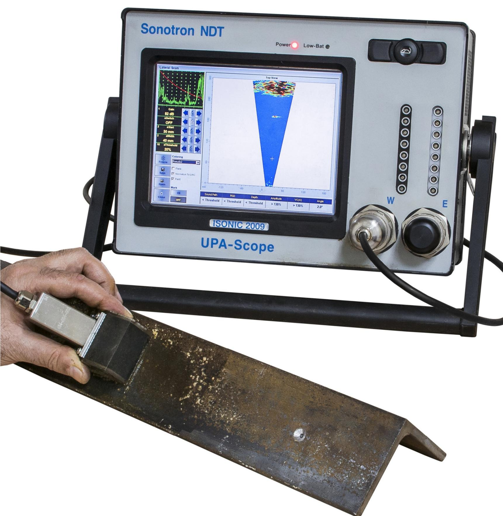
*SRUT Guided Wave Inspection with use of wedged Matrix Array Probe – the calibration block for the detection of the corrosion in the underground part of the steel poles (air to soil interface)*
