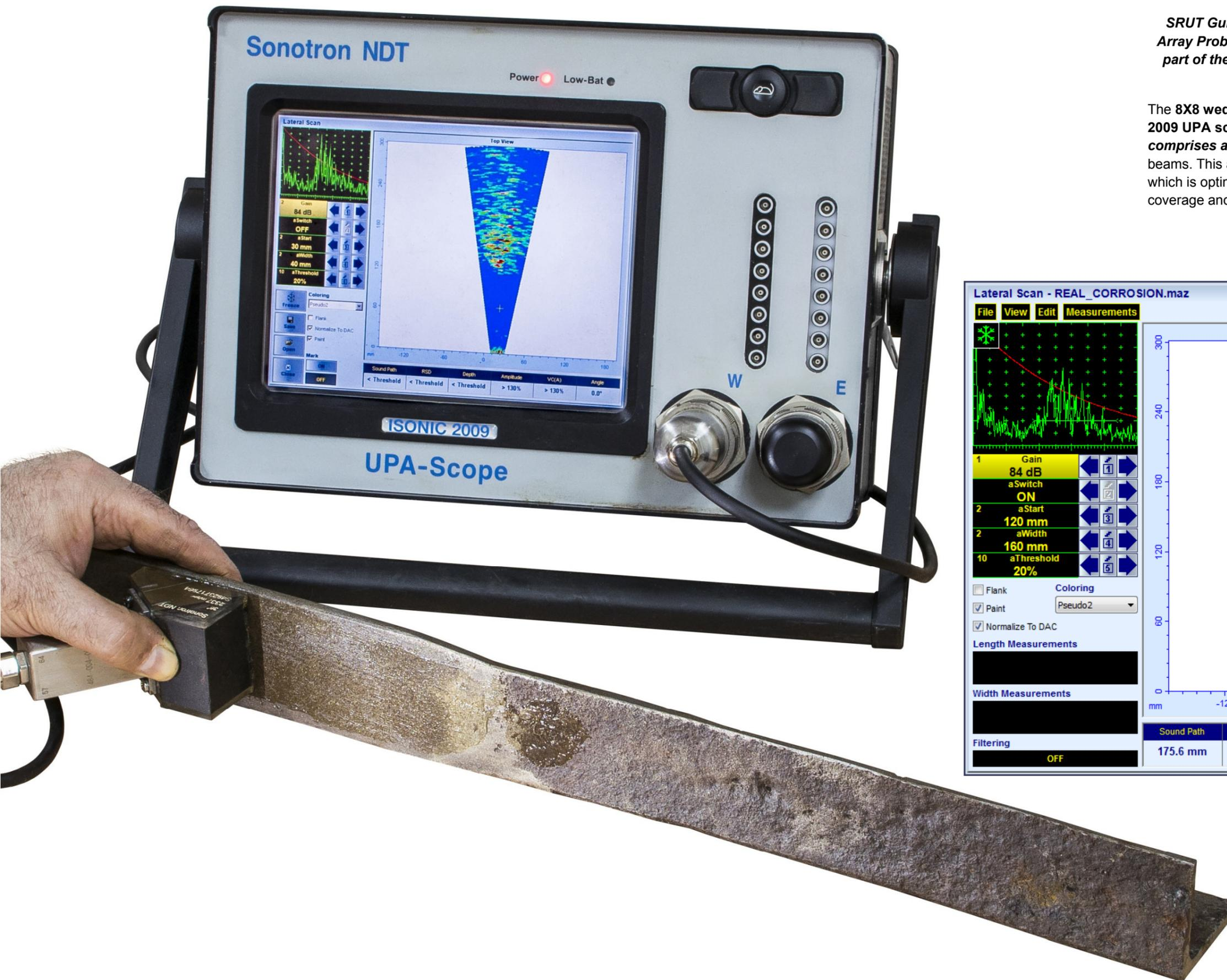
*SRUT Guided Wave Inspection with use of wedged Matrix Array Probe – detection of the corrosion in the underground part of the steel poles (air to soil interface): the cut off was taken from the real steel pole*
